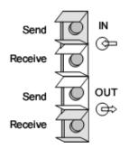
These connectors are provided for the optical waveguide between your Profibus gateway and the Profibus.
