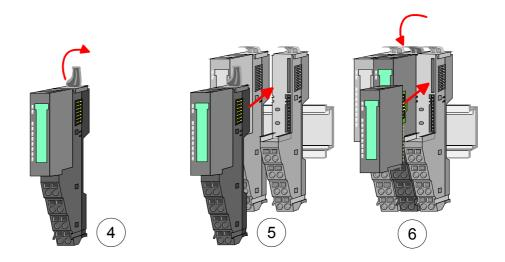
Exchange of a head module (e.g. bus coupler)
